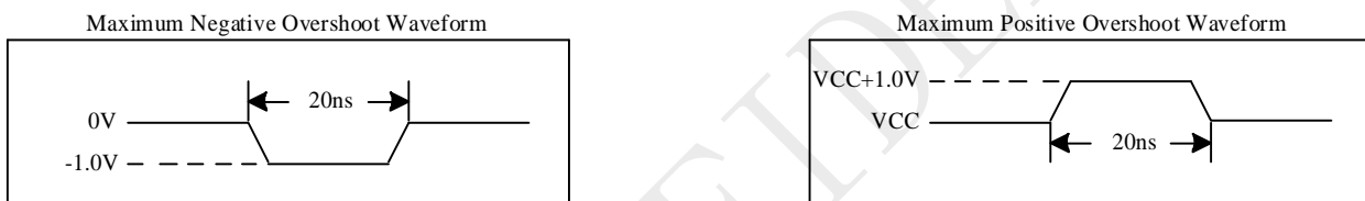
Figure 5-2 Input Test Waveforms and Measurement Level
